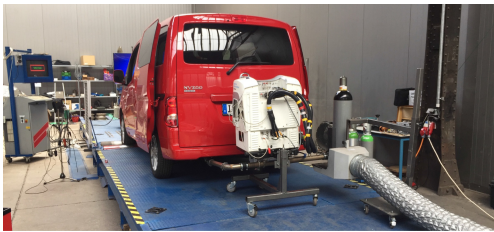
Fig. 5. Nissan NV200 Evalia on a dynamometer.
